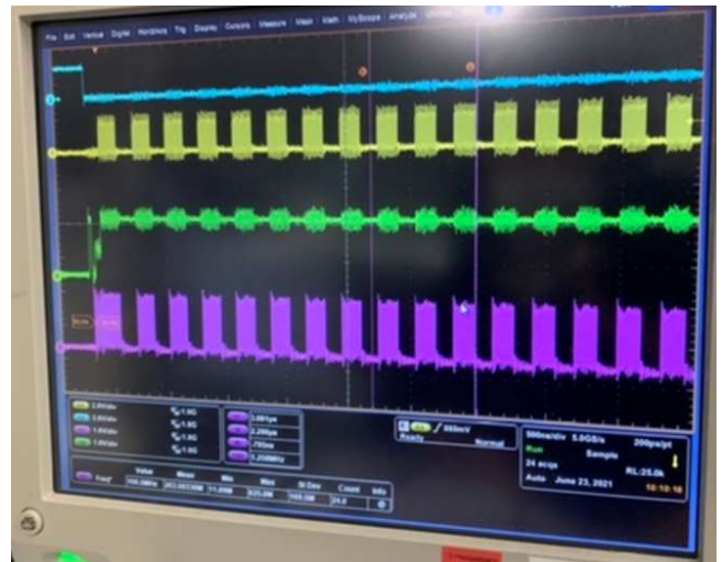
Fig. 2. Observing idle gaps on standard memcpy
